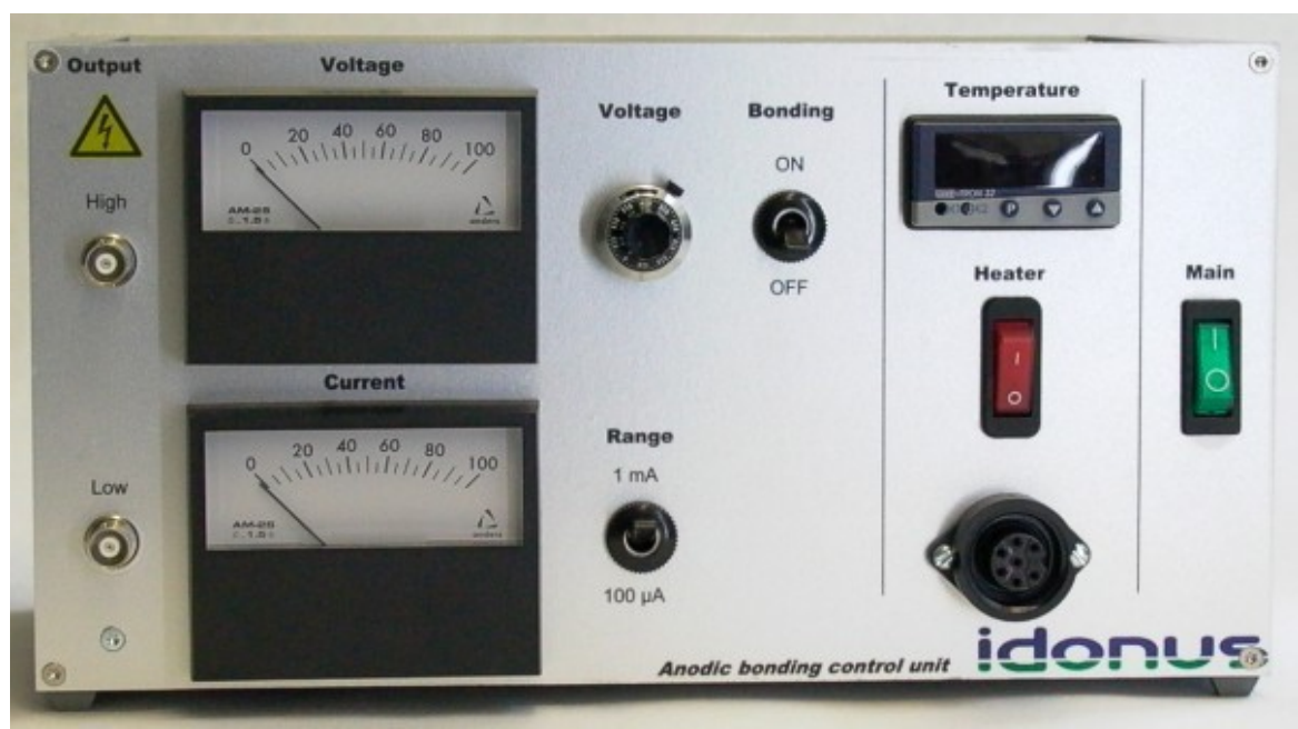
Detailed view of the controller box: The temperature controller for the heater is on the right side, the high voltage regulator on the left side. The bond-voltage and the bond-current are displayed separately.
