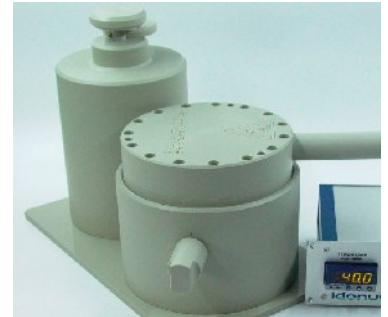
Hydrofluoric Acid Vapor Phase Etching system in operation. The reaction chamber is closed and the HF vapor remains in the chamber.
