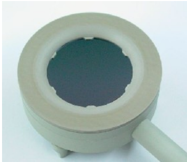
Wafer holder with mechanically clamped 100 mm wafer. The wafer is held by 6 clips to increase the etched area.
