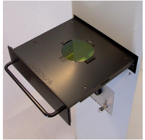
The wafer is loaded from the front side. For smaller wafers adapter rings can be used.
