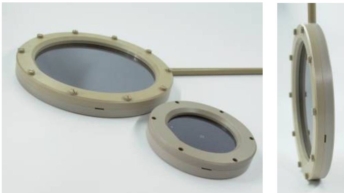
Fig. 1: Etching chuck for 100mm and 200mm wafers in PEEK (left) with ventilation tube (right).
