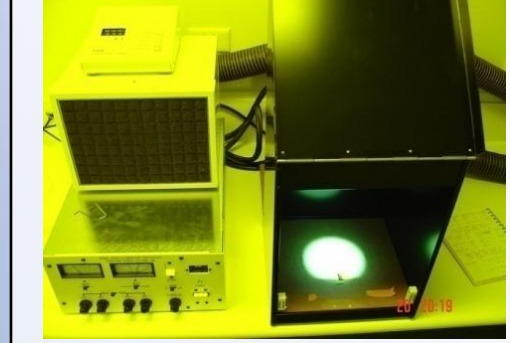
Figure 6. OAI deep UV illumination system (Model LS30/5) fitted with a 500W HgXe-lamp for the surface modification and in situ preparation of the organic polymer monolith in the polypropylene pipette tips, and photografting of reactive vinylazlactone group for trypsin immobilization.
